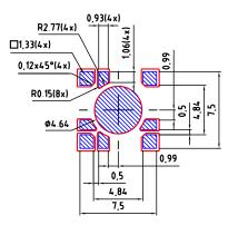
solder stencil recommended stencil thickness 200µm
