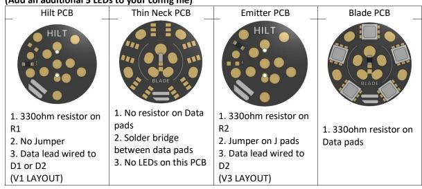
Layout 7: No Emitter LEDs but Chassis and Blade in PARALLEL
